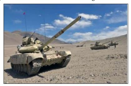
In addition, the tank has cutting-edge hybrid modular armor to make it safer. With John Cockerill's help, a complex turret was added that lets electro-optical cameras and anti-tank guided rockets be used, which increases its effectiveness.
